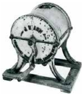
The Ash automatic ball brushing machine, c.1890, cleaned eight balls in 30 seconds!
